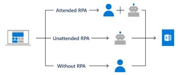
**Example 5:** Forms or data processing - An RPA triggers a macro to read information and write to systems instead of manual data entry.
